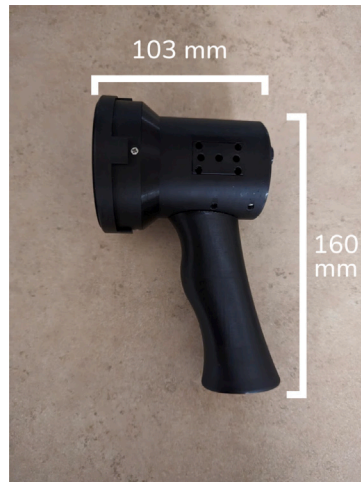
Fig. 4. The side profile of the TinyMSI with labeled height and width dimensions. Highlighting the ergonomic design of the 3D printed enclosure and the resemblance of the device to other common handheld devices like Camera Gimbals and Thermal Cameras.
